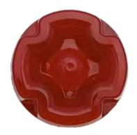
SK808F conventional siren is designed to give sound and visual warning in addressable and conventional systems. It is suitable for indoor use with its robust and stylish design. When an alarm occurs on the panel, the SK808F indoor siren becomes active and can warn people both audibly and visually. The flash on the SK808F is 360-degree visible and has a sound intensity of 86 dB (nominal) at 1 meter.
