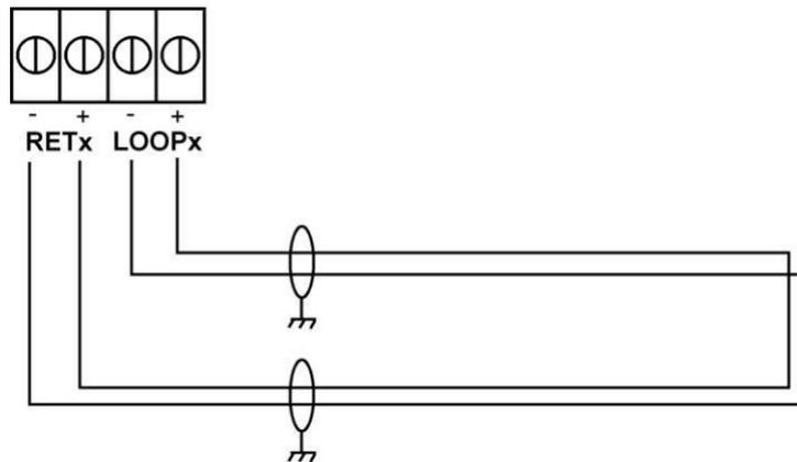
Figure 6 Loop Line Connection
