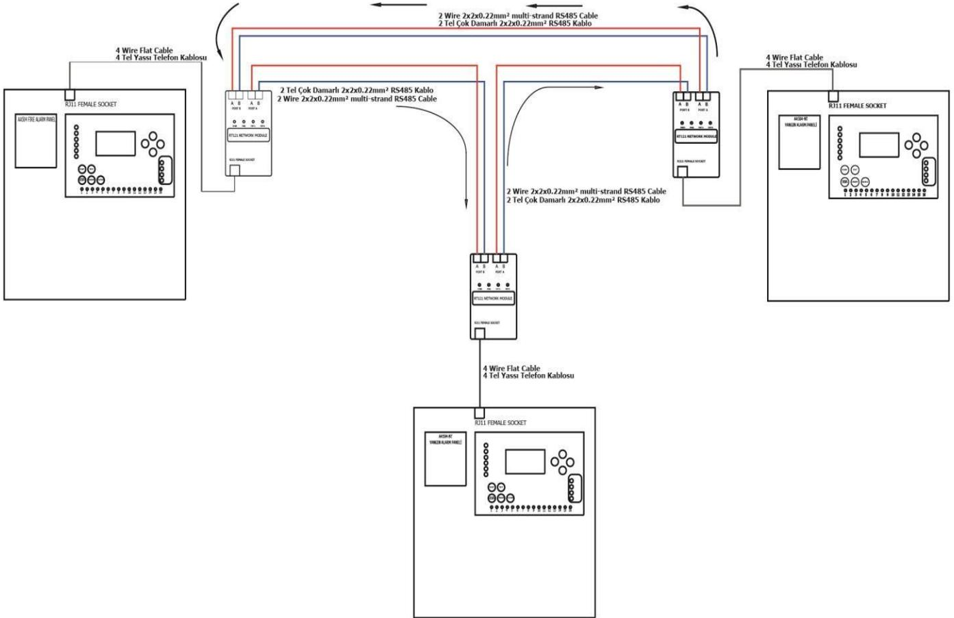
Figure 8 Network Connection Diagram
