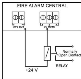
Figure 3 Open Collector Connection Diagram
