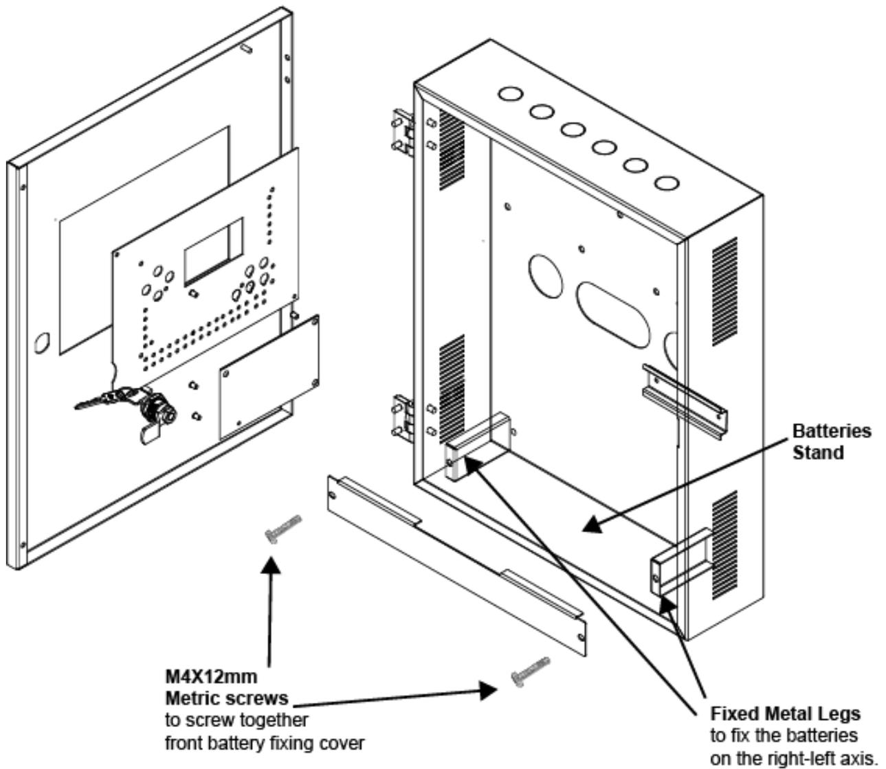
*Figure 1B Batteries Fixing Cover*
