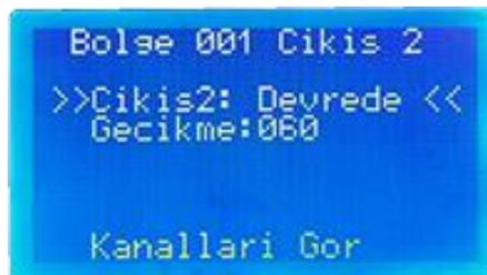
Figure 23- Output 2 Enable/Disable Screen
